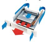
the two sides of the cover plate is emitted to the room with the assistance of different fan speeds through the central sector of the cover plate.
