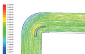
Flow lines, speed in m/s
